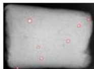
This x-ray shows a package of processed game meat. The white spots are toxic lead fragments from spent lead ammunition.
