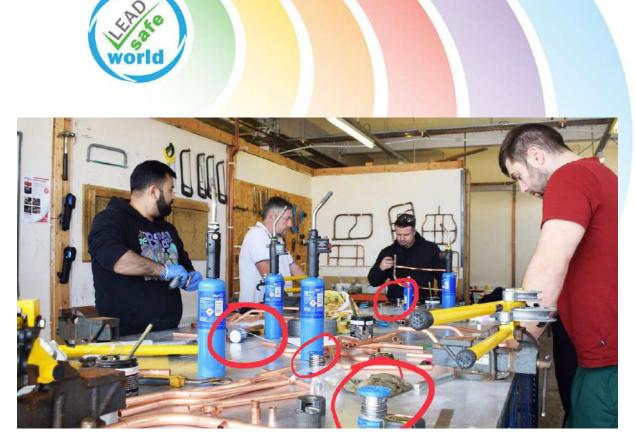
UK Further Education Colleges using lead solder - indicated by the blue/red/yellow colour of the reel (leadfree solder always has a green reel) and the grey dullness the lead solder appears when handled and soldered
