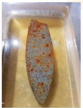
**Left:** Early Prototype after 8 weeks in salt solution of half cup of salt to 1 litre of water.
