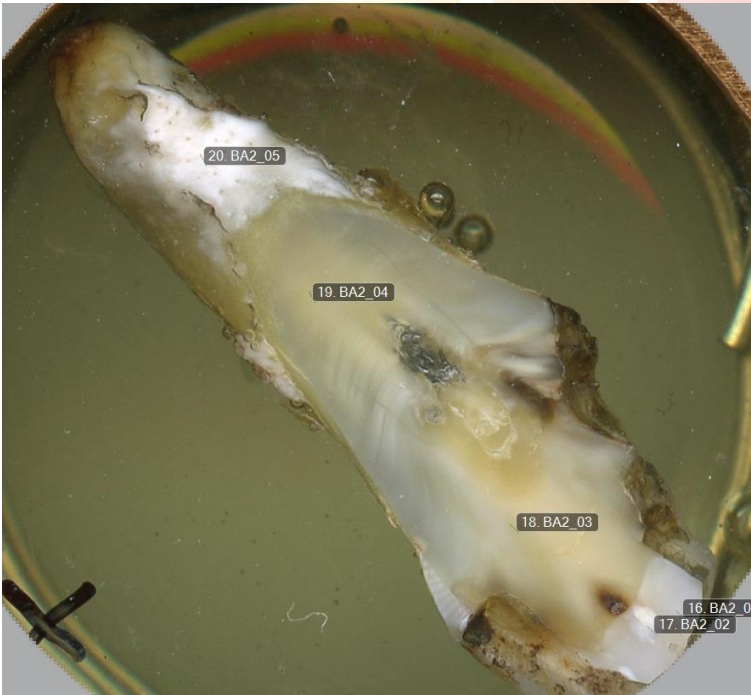
Section of Brian's incisor mounted in resin showing planned laser sampling tracks. Top BA2_01 and _02, middle BA2_03 and _04 and near root tip BA2_05. Note bright white zone in enamel may not actually be tooth material.
